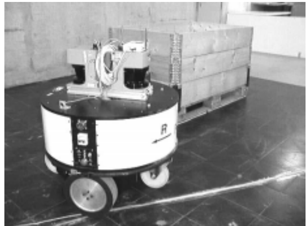
Figure 7: The robot which was used in the experiments. It is equipped with two Sick LMS200 laserscanners covering 360°. The robot is a VME based system, currently carrying a PowerPC@100MHz. It runs the deadline-driven real-time operation system XOberon. The exploration framework is implementable such that the system could execute the task in a fully autonomous mode.
