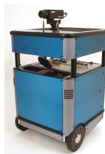
Figure 1: The autonomous robot Pygmalion. Its controller consists of a VME standard backplane with a Motorola PowerPC 604 microprocessor, clocked at 300 Mhz. Among its array of peripheral devices, the most important are the wheel encoders, a 360° laser range finder and a grey-level CCD camera.
