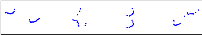
Fig. 2. Typical range readings from legs of people. As can be seen, the appearance can change drastically, also because the legs cannot always be separated. Accordingly, the proper classification of such pattern is difficult.
